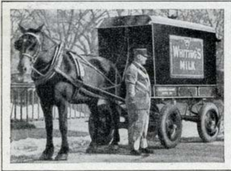
This specially-built light weight milk wagon, wearing balloon tires and drawn by horse shod with padded shoes, eliminates all clatter of milk delivery in early morning.
